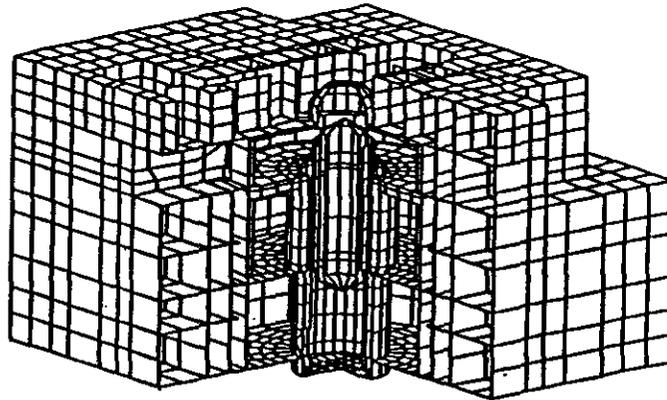
Fig. 5. Finite element model for SBWR containment and reactor building.
